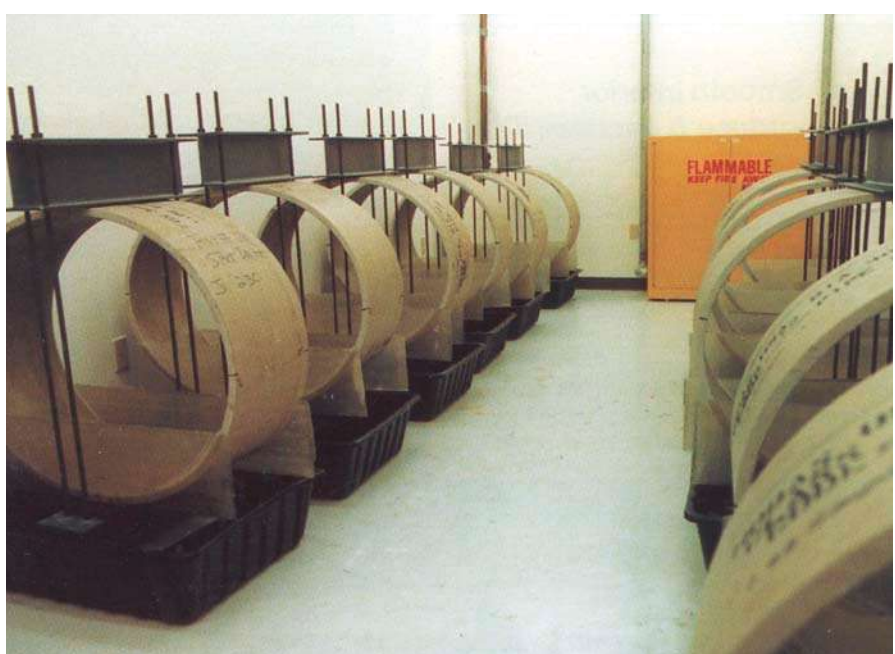
Induced ring flexural strain level tests on CCFRPM segments.
