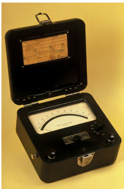
FIGURE 6. Weston DC Millivoltmeter Model 622.
