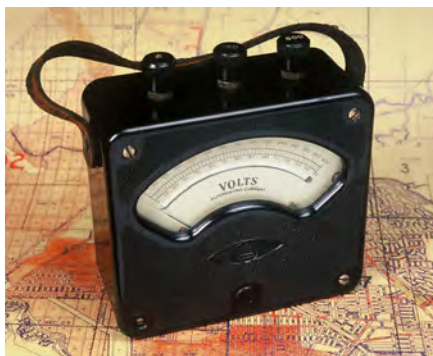
FIGURE 7. Westinghouse Electric 600-V AC Voltmeter.
