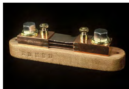
FIGURE 10. A 150-A shunt on a wood base.
