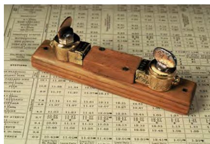
FIGURE 12. A 10-A shunt with an oak base and oak-covered resistance wire.
