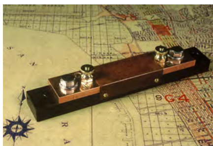
FIGURE 11. A 10-A shunt with a Bakelite base.
