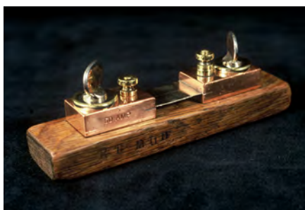
FIGURE 9. A 50-A shunt on an oak base.
