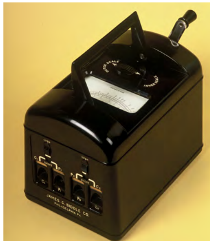
FIGURE 22. Megger Ground Resistance Meter Model CVM.
