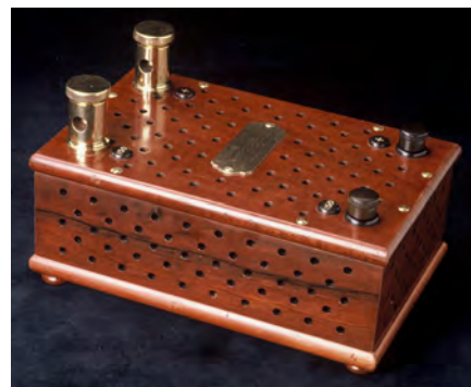
FIGURE 8. A nineteenth-century 150-A DC shunt.
