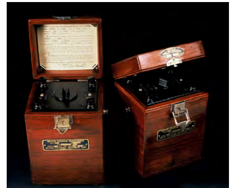
FIGURE 25. Weston potential transformers housed in walnut cases.
