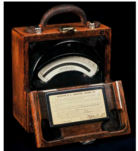
FIGURE 4. Weston DC Ammeter Model 45.
