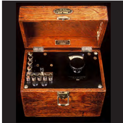
FIGURE 20. Leeds & Northrop Potentiometer.
